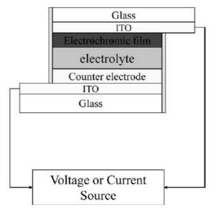
**Fig. 1.** Five-layer electrochromic device scheme composed of a glass-ITO substrate (GS-TC), electrochromic (EC) and counter electrode (IS) films and electrolyte (IC).
